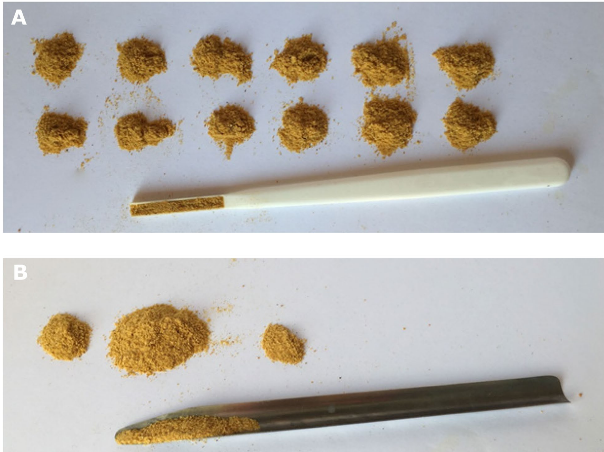
Figure 6. Increments from a uniform 1- or 2-dimensional slab cake. (A) Equal/proportionate increments, resulting in control of increment weighting error (IWE). (B) Unequal/disproportionate increments, resulting in uncontrolled IWE. © Lawrence Novotny and Nancy Thix (Thix Laboratory Solutions LLC, Brookings, South Dakota).
