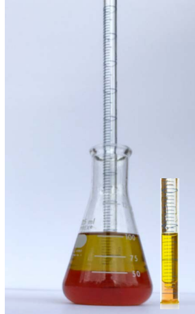
Figure 8. Examples of correct and incorrect increment delimitation: (A) open tube in a multiphase liquid (olive oil and red wine vinegar) in a cylinder; (B) open tube in a multiphase liquid (olive oil and red wine vinegar) in an Erlenmeyer flask.
