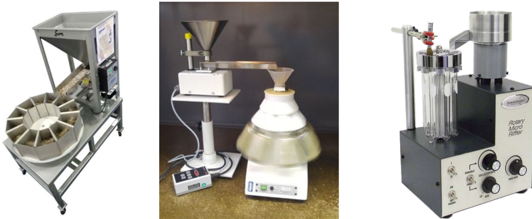
Figure 13. Examples of rotary splitters, ranging from large-capacity floor model to medium-capacity bench top to micro-capacity bench top.
