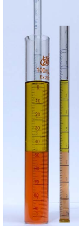
Figure 8. Examples of correct and incorrect increment delimitation: (A) open tube in a multiphase liquid (olive oil and red wine vinegar) in a cylinder; (B) open tube in a multiphase liquid (olive oil and red wine vinegar) in an Erlenmeyer flask.
