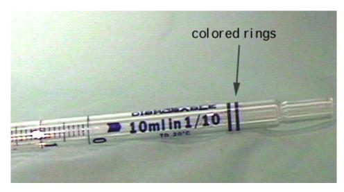
• A pipette is calibrated with a series of graduation lines to allow the measurement of more than one volume. Measure using the bottom of the concave surface of the liquid in pipette. This figure illustrates how to read the meniscus on a measuring pipette.
