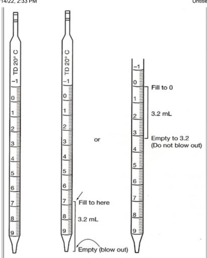
The bands at the top indicate that this pipette is to be "blown-out."
